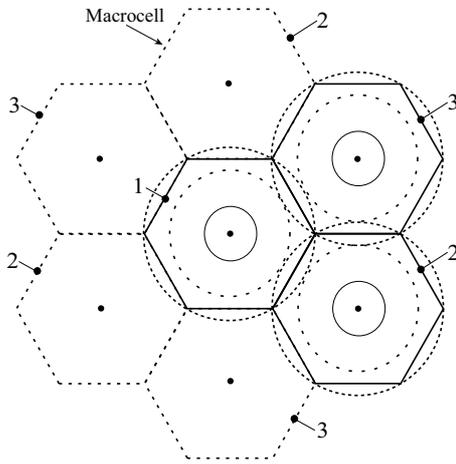
Fig. 6. An illustration of single macrocell coverage. The demonstration of a super macrocell arrangement. The number of each macrocell is denoted as a different identification of  $C_h$ , which is reserved to avoid interference and co-channel effect with each other.
