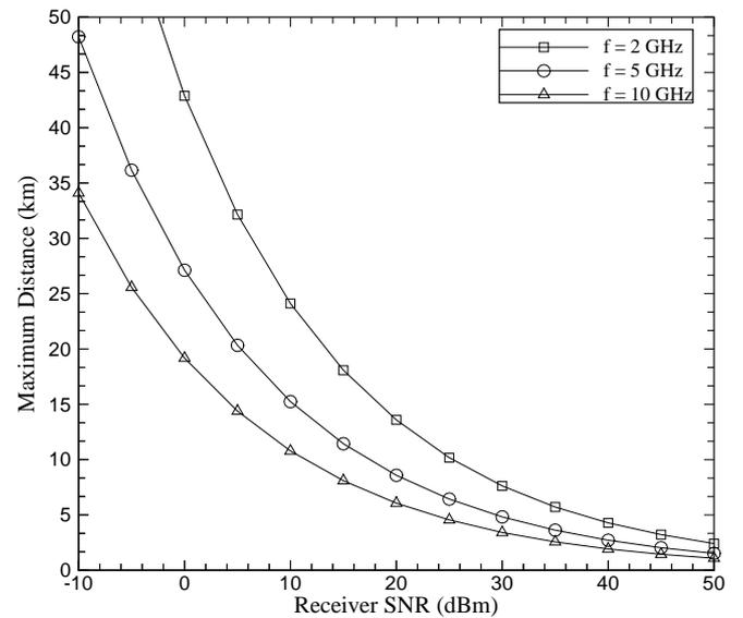
Fig. 4. Maximum distance versus receiver SNR when  $\sigma = 4$ ,  $B = 20$  MHz, coding rate =  $3/4$ ,  $F = 7$ ,  $G_t = 15$ ,  $G_r = 18$ ,  $P_t = 15$  W,  $L = 5$  dB.
