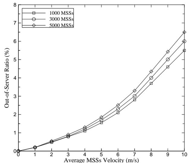
Fig. 12. The out-of-service ratio versus average velocity of the MSS when  $M = 1000, 3000,$  and  $5000$  by using SDCA.
