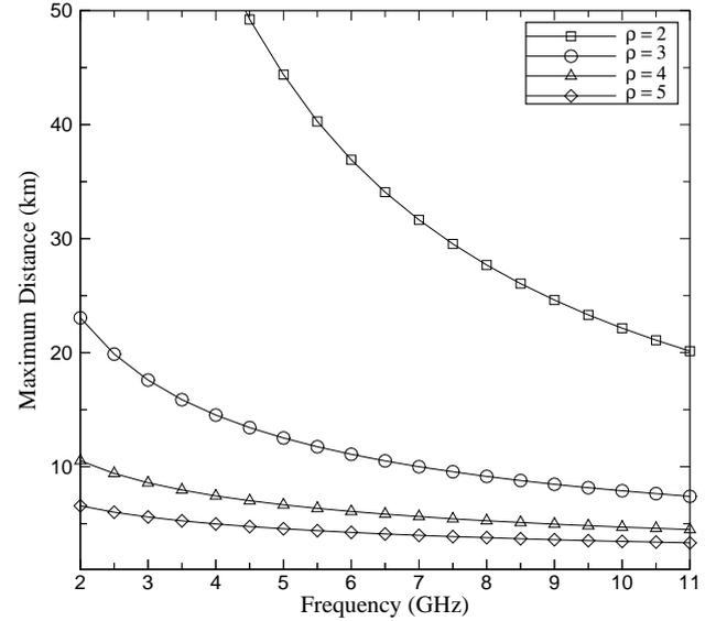
Fig. 3. Maximum transmission distance versus frequency when  $B = 20$  MHz, coding rate =  $3/4$ ,  $\text{SNR}_{r,\min} = 24.4$  dB,  $F = 7$ ,  $G_t = 15$ ,  $G_r = 18$ ,  $P_t = 15$  W,  $L = 5$  dB.
