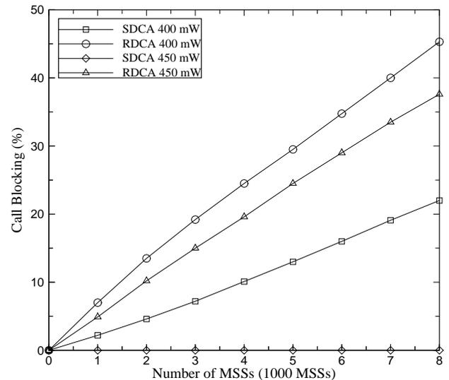
Fig. 11. The Call blocking ratio versus different number of MSSs under the maximum transmission power.
