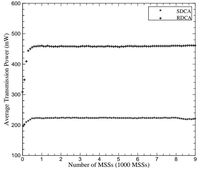
Fig. 9. The average transmission power versus the number of MSSs ( $M$ ) when  $\sigma = 4$ ,  $B = 5$  MHz, coding rate = 3/4,  $SNR_{r,min} = 24.4$  dB,  $F = 7$ ,  $G_t = 16$ ,  $G_r = 18$ ,  $L = 5$  dB.
