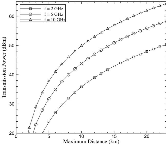
Fig. 2. Transmission power versus maximum distance when  $\sigma = 4$ ,  $B = 20$  MHz, coding rate =  $3/4$ ,  $\text{SNR}_{r,\min} = 24.4$  dB,  $F = 7$ ,  $G_t = 15$ ,  $G_r = 18$ ,  $L = 5$  dB.
