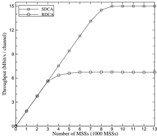
Fig. 10. The comparison of channel throughput derived by SDCA and RDCA when number of MSSs nodes.
