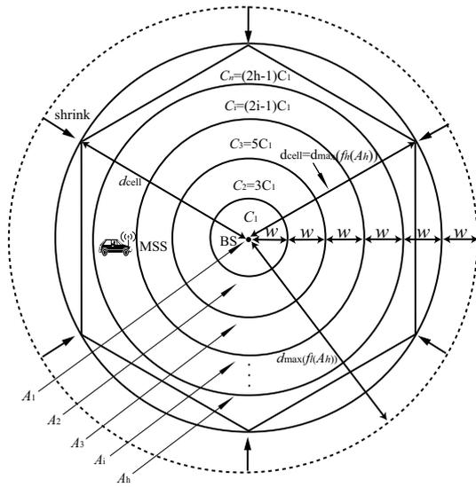
Fig. 5. An illustration of channel arrangement within the macrocell in a three-dimensional way. The channel allocation is from highest frequency to lowest frequency and is started from the inner side of the macrocell (the left side of the figure).
