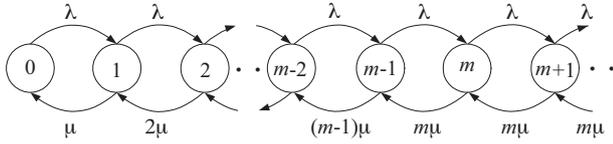
Fig. 5. The rate transition diagram for the M/M/m queue.
