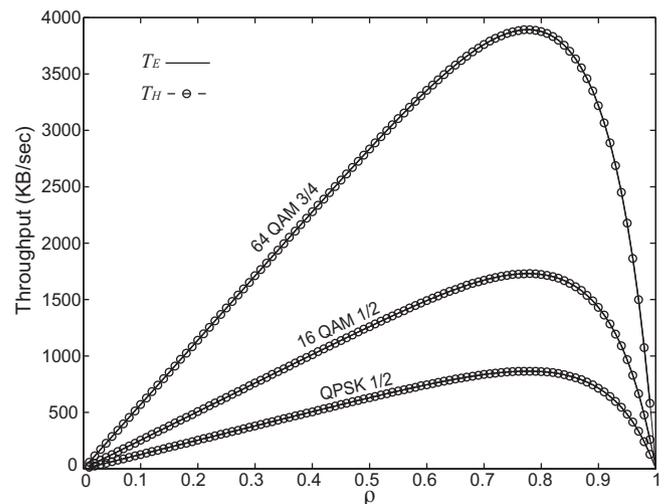
Fig. 9. The uplink throughput vs. work load  $\rho$  when  $m = 11, k = 24, N_s = 18,$  and  $\mu = 24/18$ .
