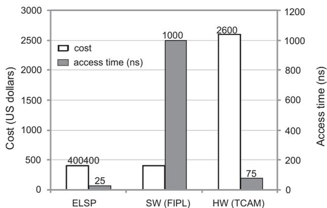
Fig. 14. Cost vs. access time at three mechanisms.
