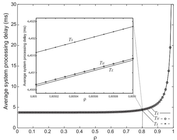
**Fig. 6.** Average processing delay vs. work load  $\rho$  when  $m = 11$ ,  $k = 24$ ,  $\ell = 18$ , and  $\mu = 1.33$  with the transmission rate 16-QAM 1/2.
