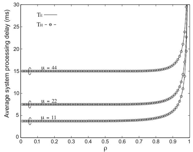
Fig. 8. Average processing delay vs. work load  $\rho$  under different  $m = 11, 22,$  or  $44$  and  $\mu = 24/18, 12/18,$  or  $6/18$  when  $N_s = 18$ .
