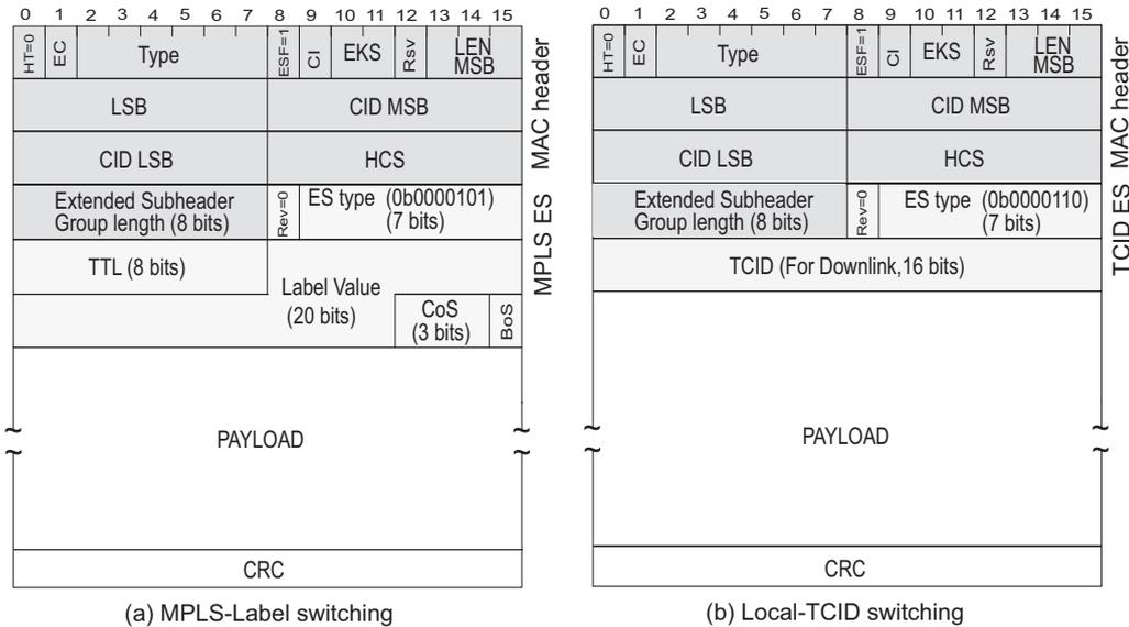
**Fig. 2.** The standard IEEE 802.16e data frame header format with subheader extension: (a) the new subheader extension of M-label with ES type coded as 0b0000101 and (b) the new subheader extension of local TCID number with ES type coded as 0b0000110.
