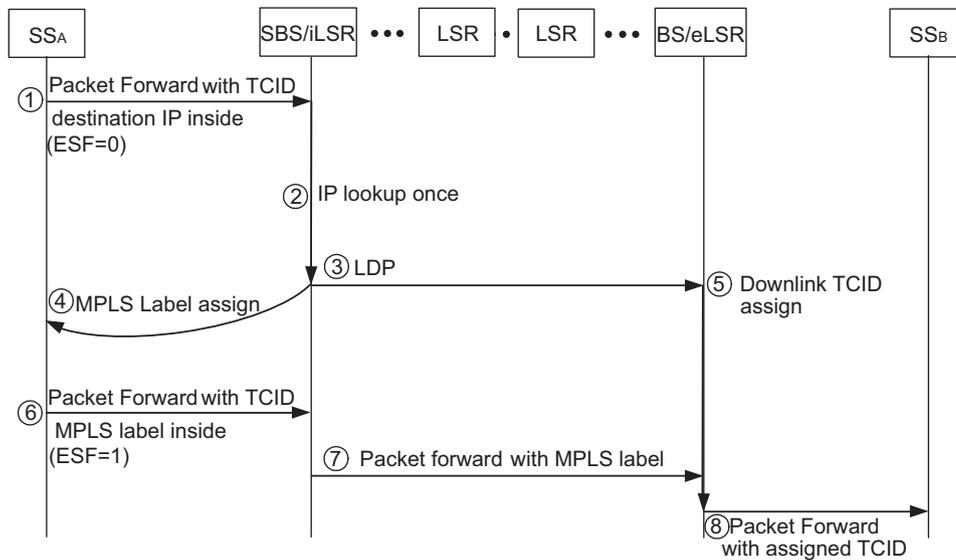
Fig. 3. The transmission identification process of outgoing traffic in the ELSP.
