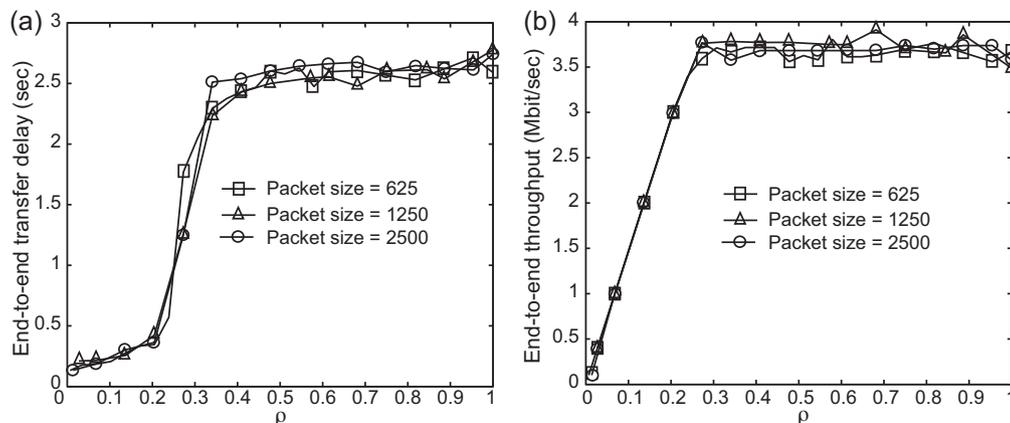
Fig. 13. The comparisons of the end-to-end transfer delay and throughput in terms of two SSs to two SSs transmission over WiMPLS networks when  $m = 11, k = 24$ , and  $\mu = 24/18$ .
