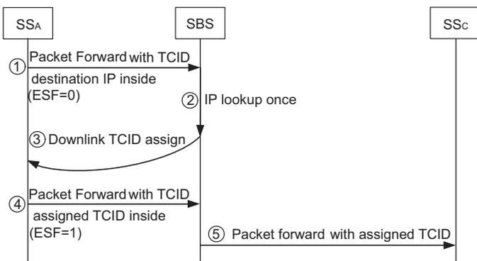
Fig. 4. The transmission identification process of local traffic in the ELSP.
