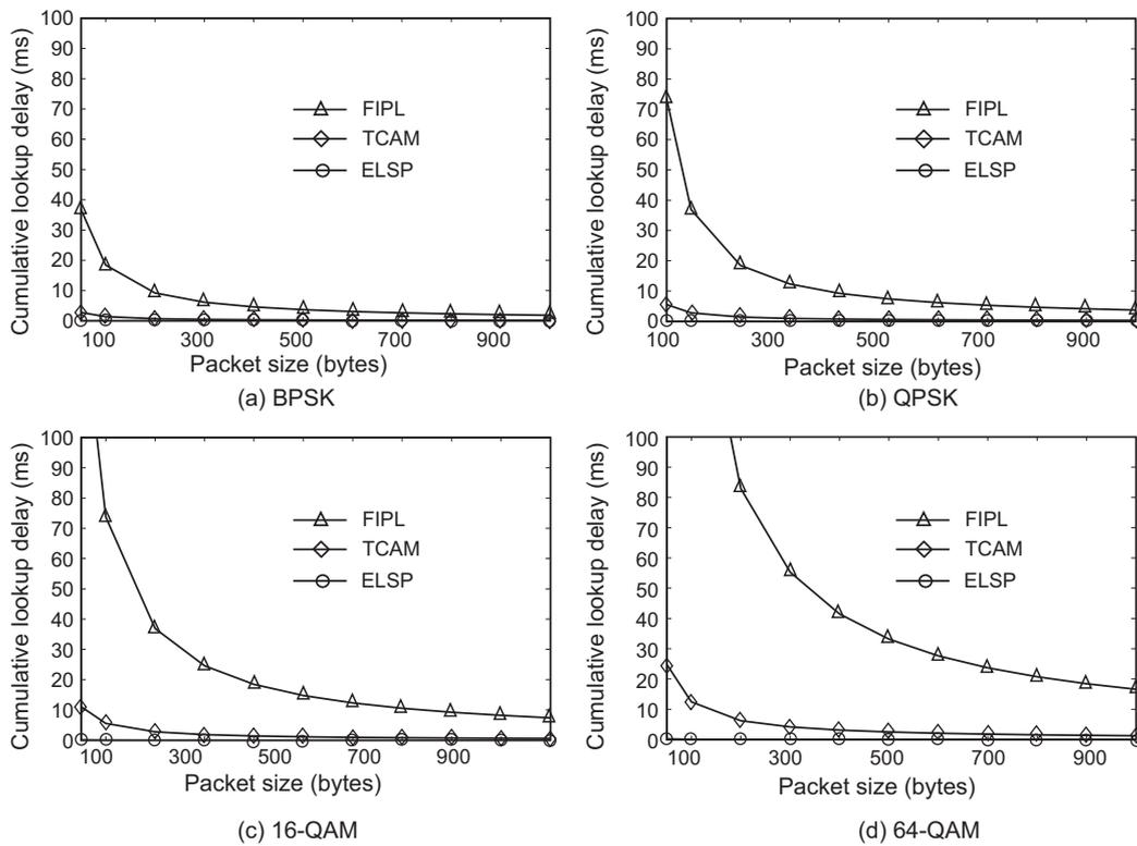
Fig. 10. The comparisons of the cumulative IP lookup delay vs. the packet size by different modulation schemes.
