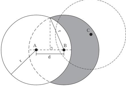
Figure 4: Analysis of the impact of hidden terminal problem: station A sends a packet and station B received the packet.
