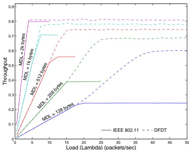
Figure 6: Comparison of throughput of IEEE 802.11 and DFDT with different MDLs when  $N = 25$  and  $CT = 2312$  octets.
