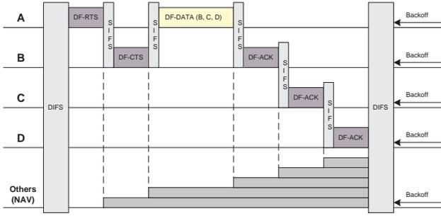
Figure 3: The mechanism of DFDT (In this diagram the data frame is compiled from three data packets).
