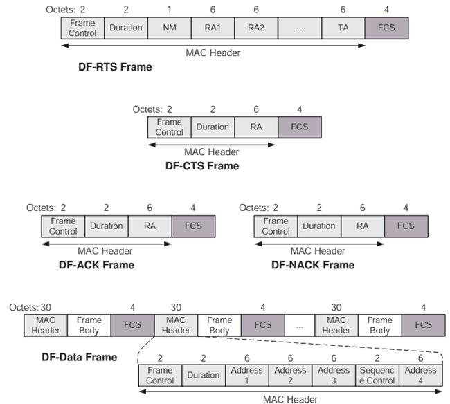
Figure 2: The frame format of DFDT.
