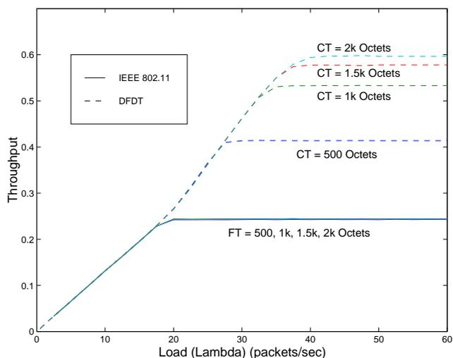
Figure 7: Comparison of throughput of IEEE 802.11 and DFDT with different CT and FT values when  $N = 25$  and MDL = 128 octets.
