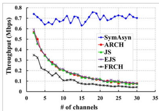
Fig. 12. Throughput versus number of channels.
