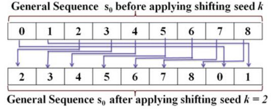
Fig. 5. Example of left circular Shift by  $k = 2$ .
