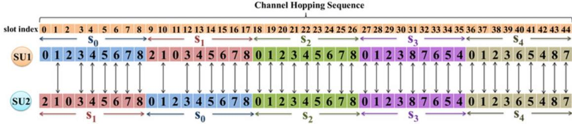
Fig. 4. Rendezvous between two secondary users (SUs) in symmetric synchronous environment.
